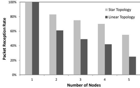
**Figure 3. Network behavior: packet reception rate for linear and star topologies when more nodes are added into the simulated network.**
