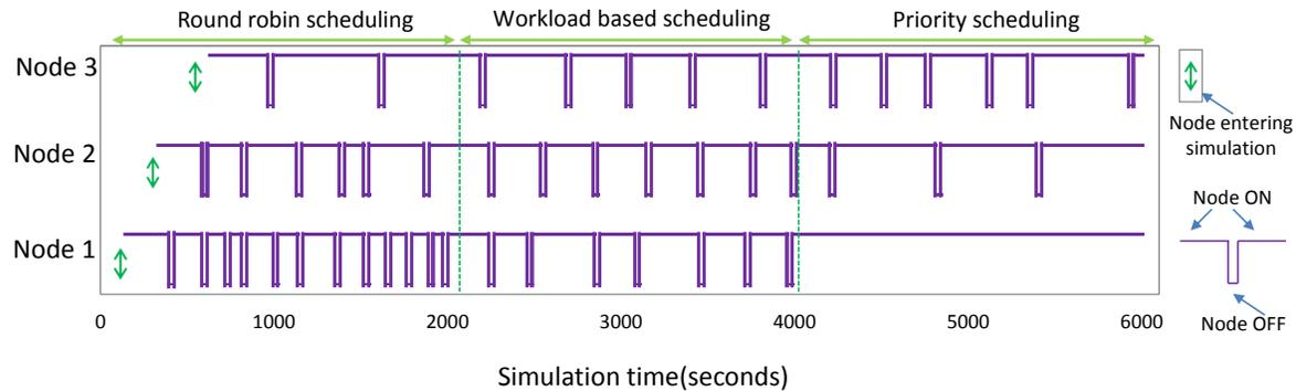
**Figure 4. Impact of different energy scheduling algorithms on node and network behavior.**
