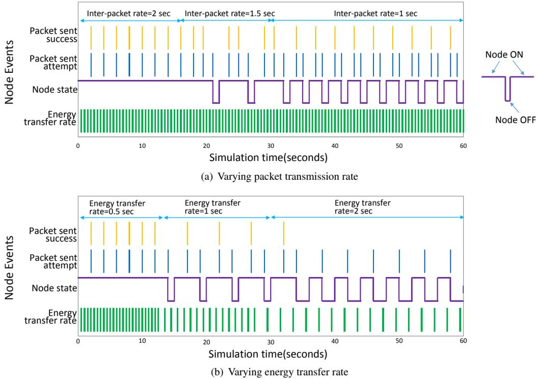
**Figure 2. Node behavior: frequent shutdowns and reboots occur either by increasing the workload or by decreasing the recharging rate.**
